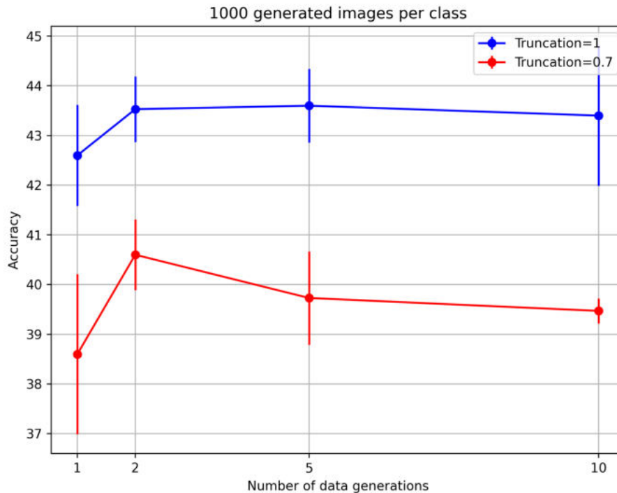
Figure 4.11: Performance comparison between different synthetic dataset generation strategies on Imgewoof. It can be seen that repeated data generation does not benefit the overall performance while increasing the training time significantly. This motivates us to generate data for downstream tasks only once - prior to the training.
