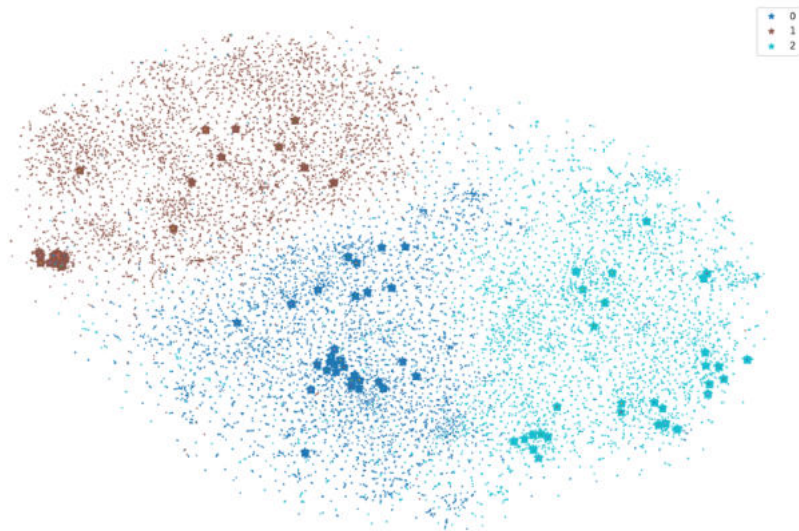
Figure 4.15: TSNE illustration of different initializations. In the Figure can be seen the TSNE plot of the first 3 CIFAR10 classes and images selected for initialization are marked with stars. We can observe that High entropy initialization (upper) concentrates on borders between classes, where hardest-to-classify samples are, while low entropy initializations (bottom) are mostly clustered in high confidence areas.
